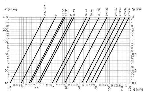
The maximum recommended flow speed at the device connections is  $\sim 1.2$  m/s.
