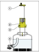
When checking the internal element of threaded deaerators and dirt separators, simply unscrew the large dirt collection chamber (5) to which the internal element is fixed, so that it can be removed for cleaning.
